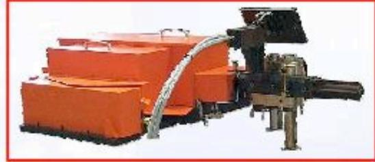
EGD450 is a high performance Gob Distributor system for IS Machines, available in "stand alone" or COMBI version (with the FMC450 Drive system or EPS120Pusher system). In the COMBI version the two systems will be housed in the same cabinet.
